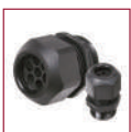
Cable Gland Multi Hole Heyco® Tite Liquid Tight Cordgrips for Multi Hole Application Cable ø 1,4 – 4,0 mm Thread: NPT, PG, Metric UL, CSA, VDE, NEMA Approval
