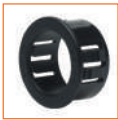
Bushing, SNAP-IN for Material Thickness to 6,4mm Nylon Heyco® Thick Panel Snap Bushings Mounting Hole \varnothing 9,5 – 50,8mm UL, CSA Approval
