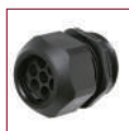
Cable Gland Multi Hole Heyco® Tite Liquid Tight Cordgrips for Multihole Application Cable ø 4,2 – 9,5 mm Thread: NPT, PG, Metric Integrated Sealing ring, UL, CSA, VDE, NEMA Approval
