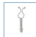
HEYClip™ Lockit™ Loops with Standoff Blind Mount, SNAP-IN Cable Bundle ø 7,0 – 15,0mm Mounting Hole ø 7,9mm UL-Approval
