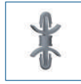
PCB Spacer - SNAP-IN Heyco® Nylon PCB Support Mounting Hole ø 4,0-4,8mm UL-Approval
